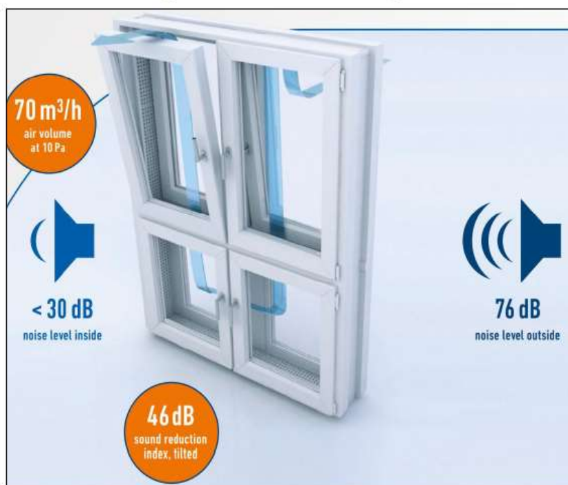
Figure 15. Plenum Window Example 2
