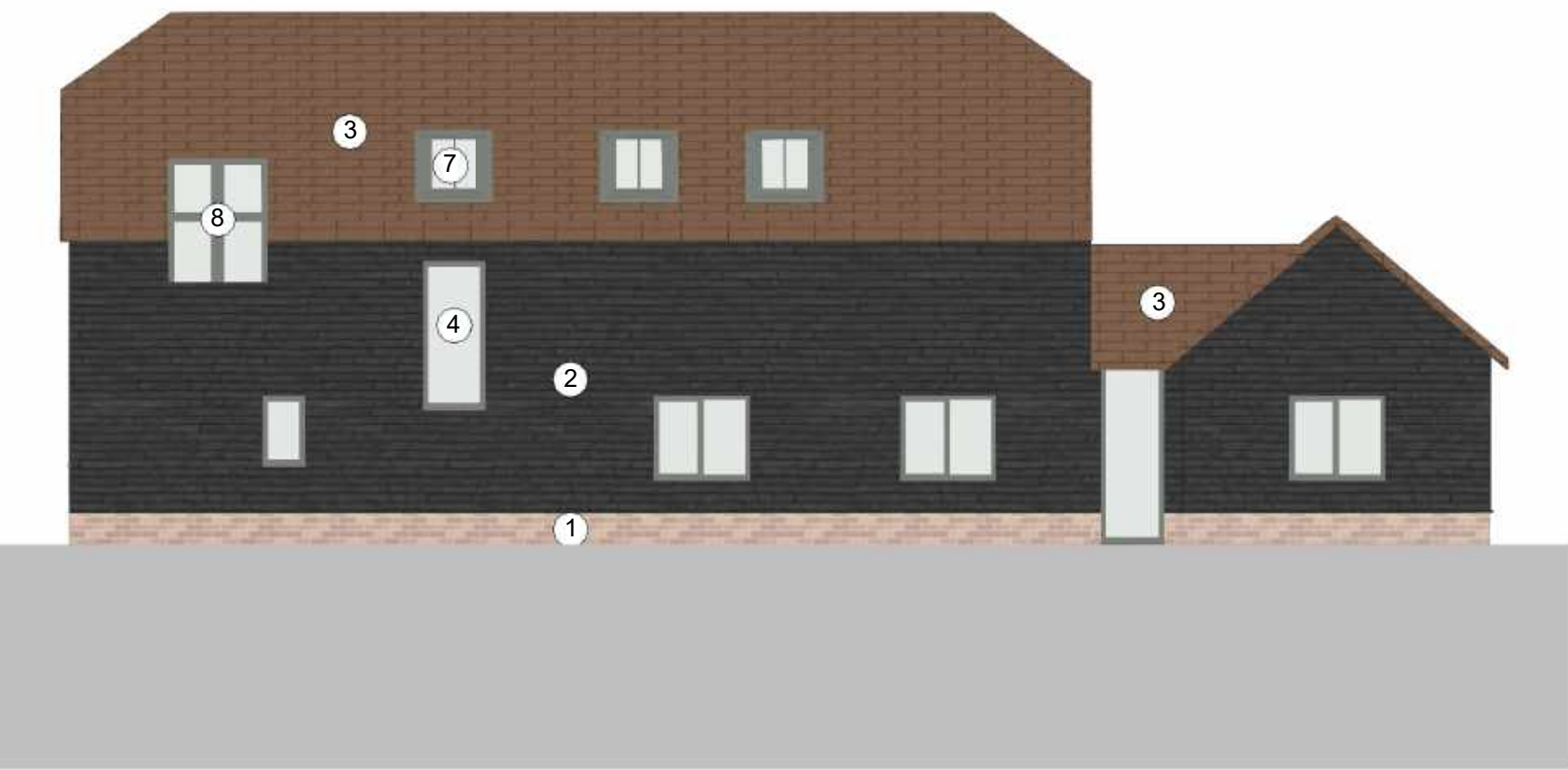
5 Elevation - North Main House 1 : 100
