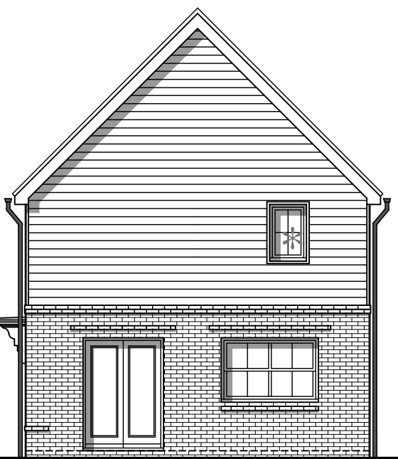
SIDE ELEVATION * OBSCURE GLAZED WINDOWS
