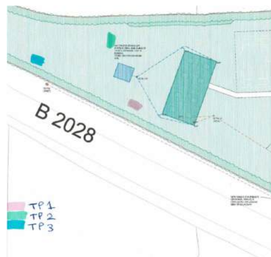
Figure 8: BRE365 soakage test locations
