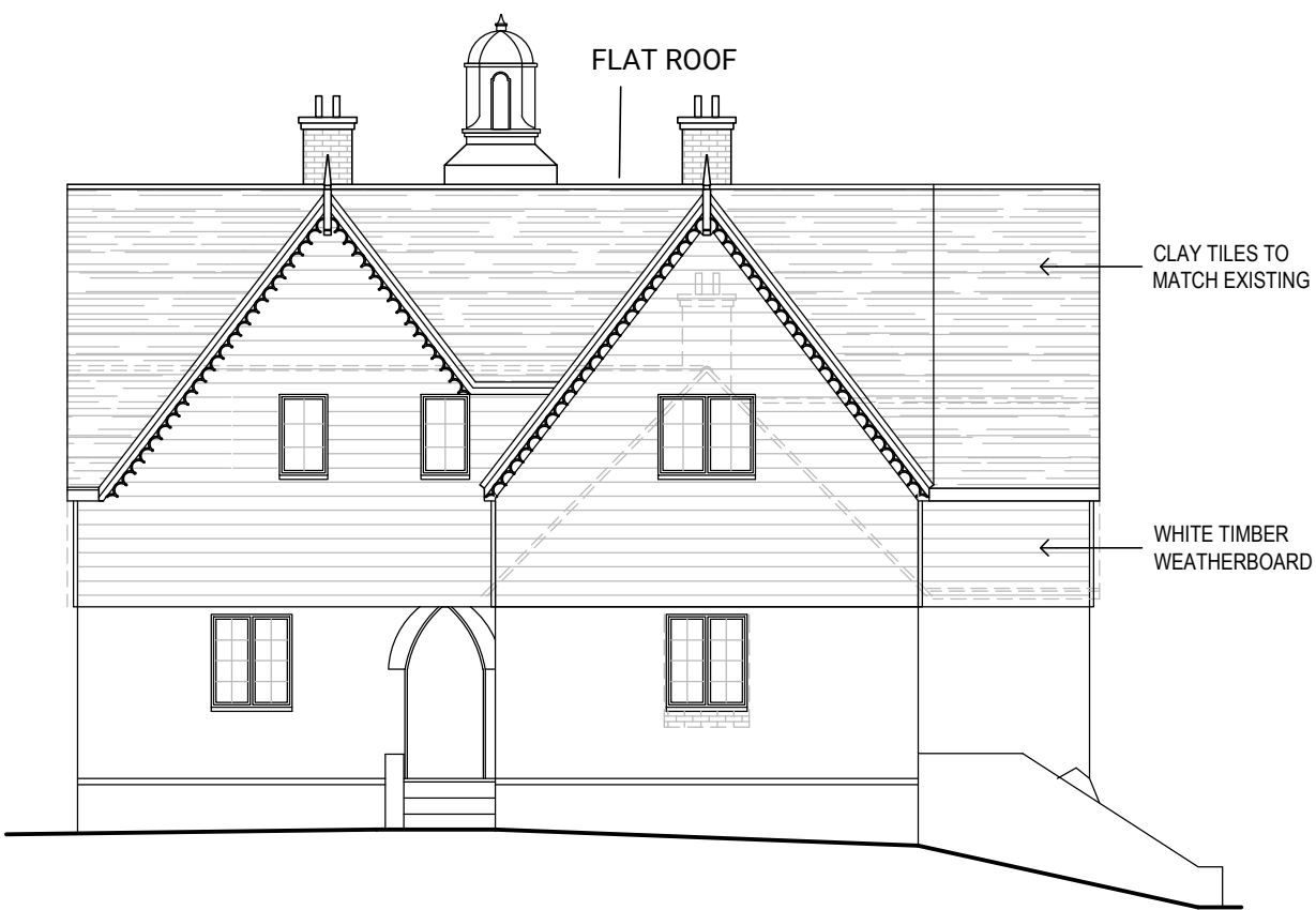
FRONT ELEVATION North
