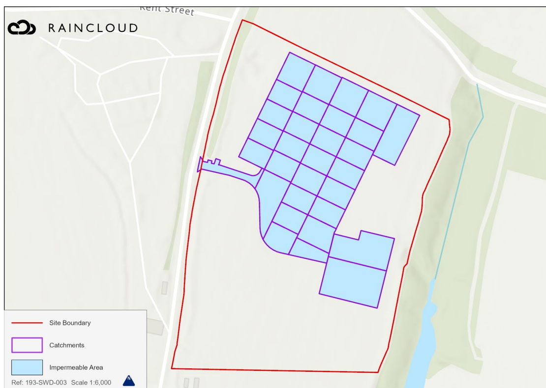
Figure 3: Catchments and Impermeable Areas
