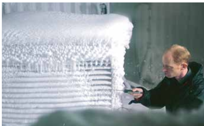
Climatic chambers simulate all possible operating conditions
