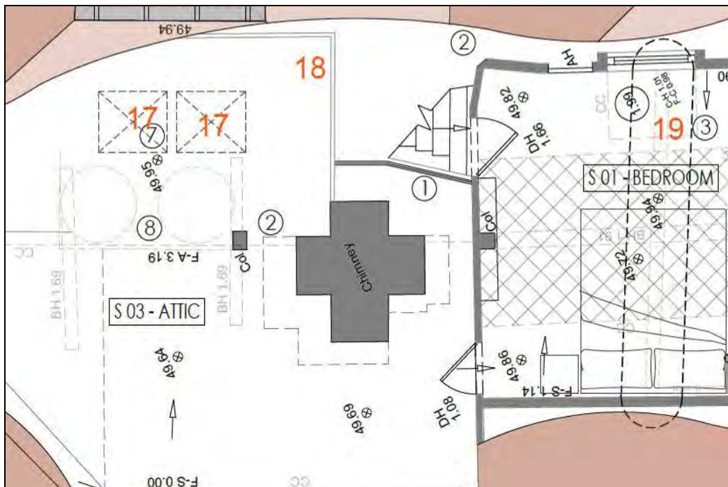
Plate 52: New partitions proposed in bay 3, east side
