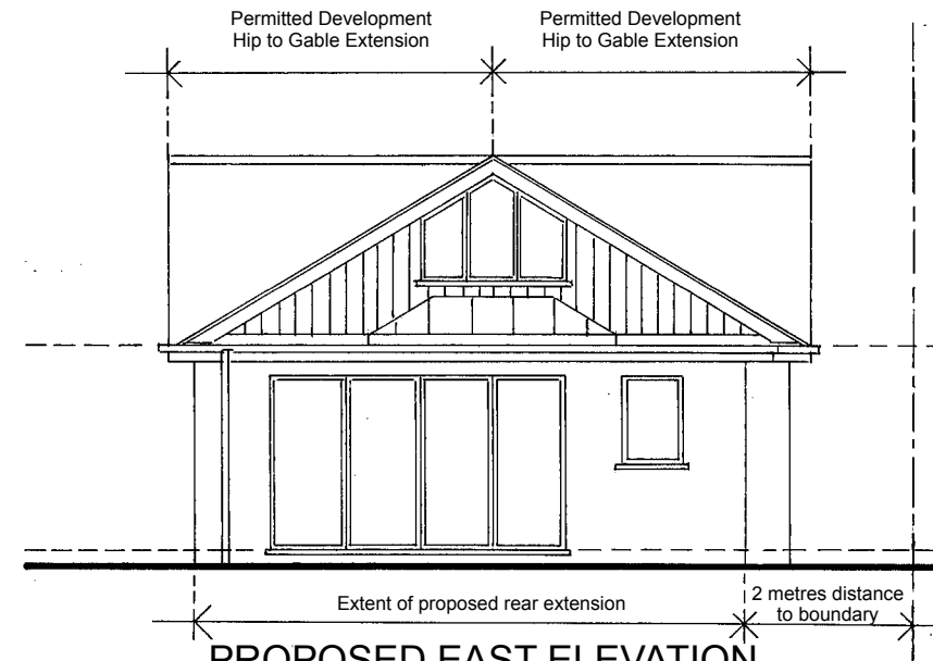
PROPOSED EAST ELEVATION
