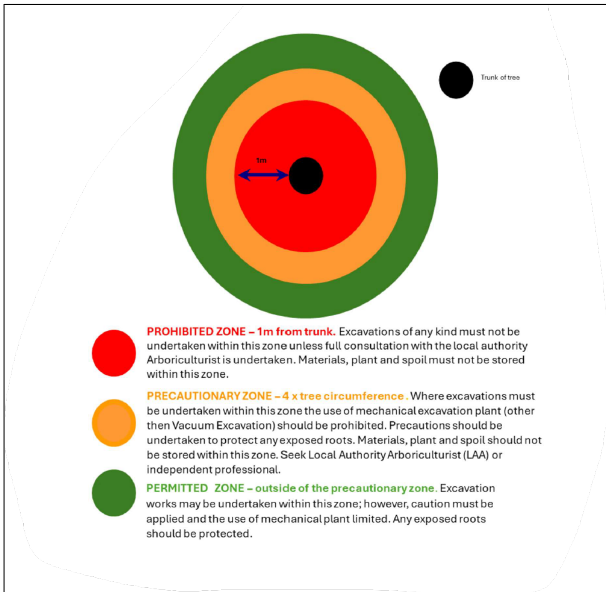
Figure 4: showing a summary of the three zones around trees in relation to underground utilities 8 .
