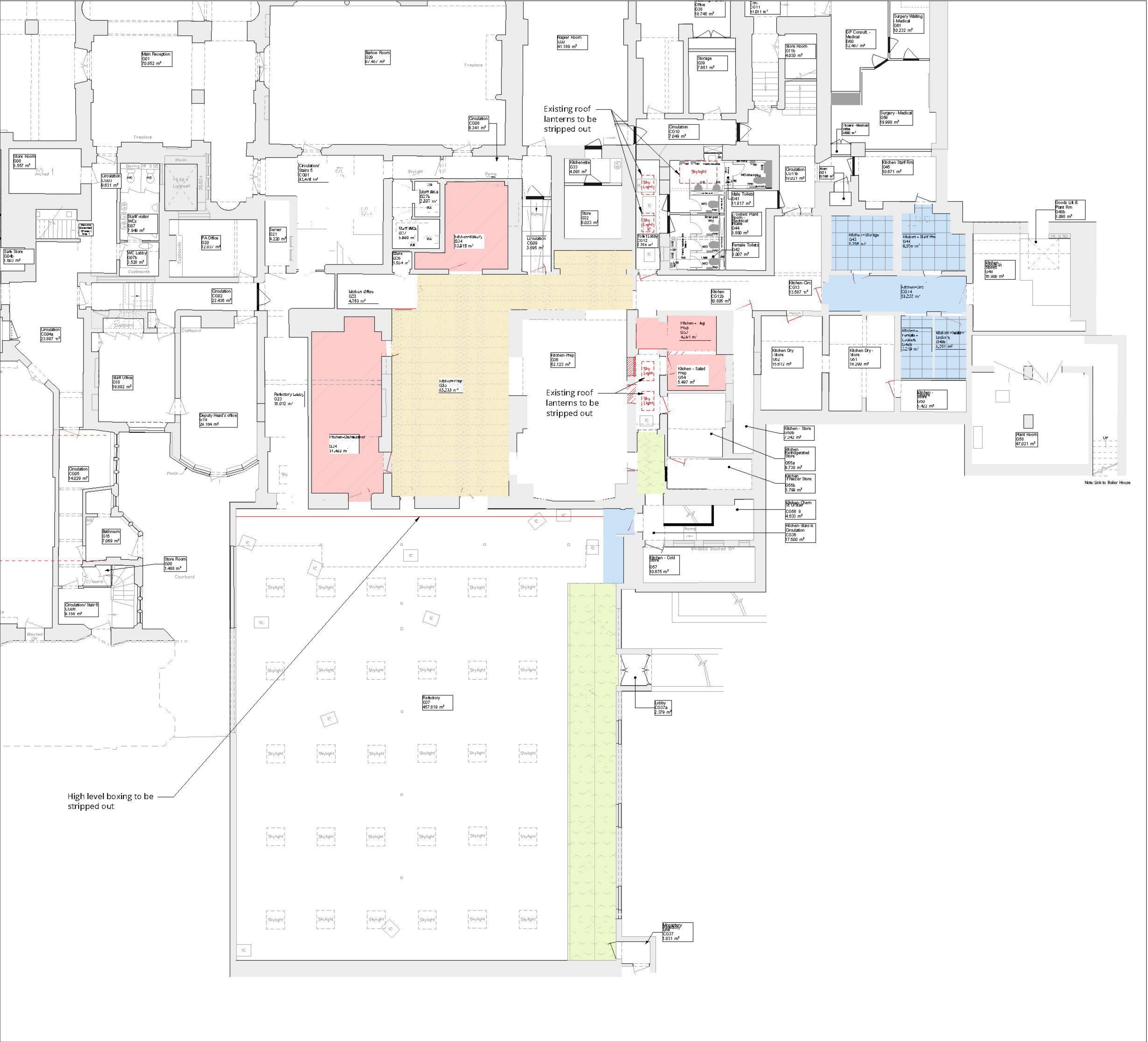
PROPOSED ALTERATIONS TO CEILINGS to Ground Floor Plan Scale 1:100
