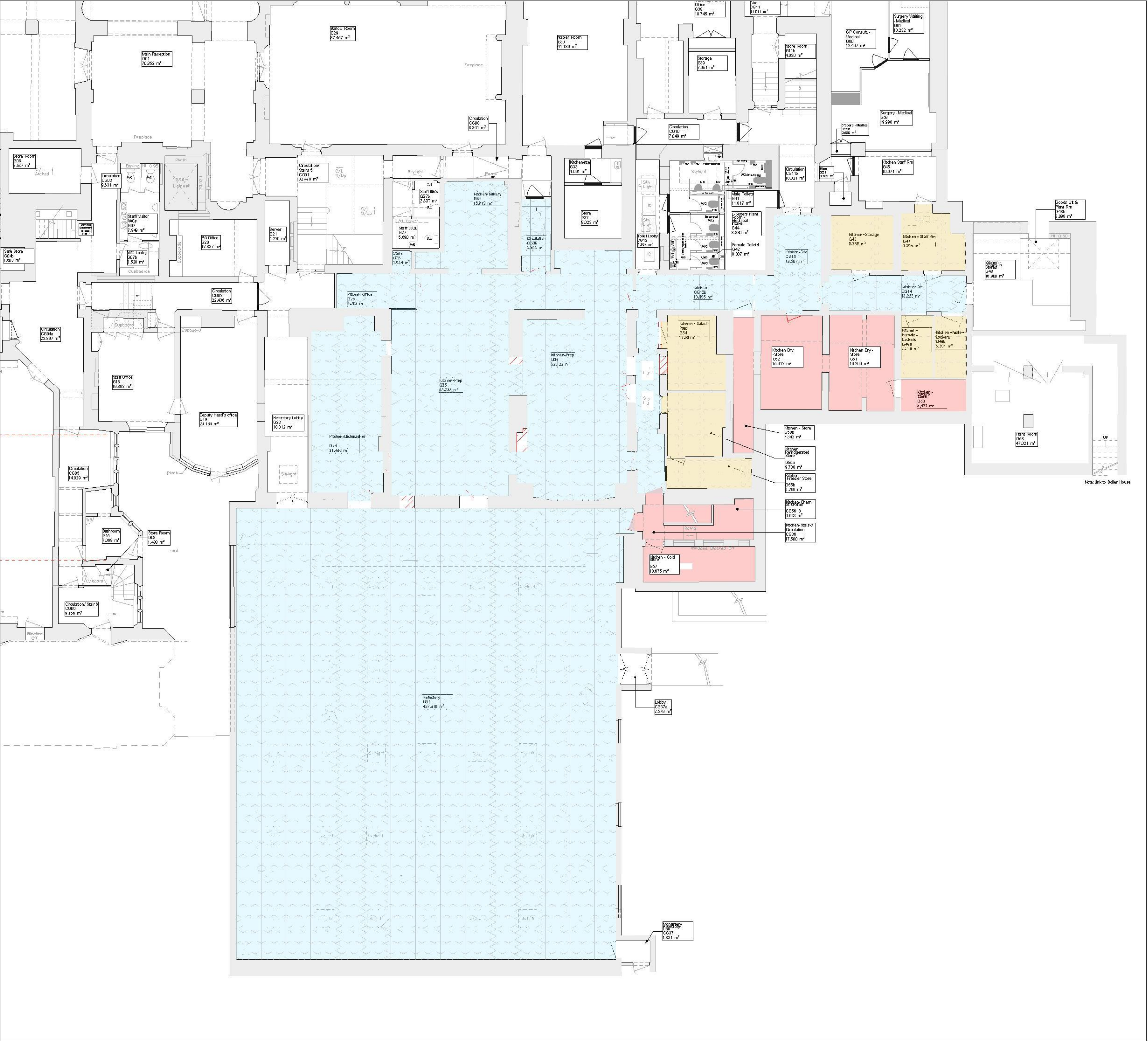
PROPOSED CEILINGS to Ground Floor Plan Scale 1:100
