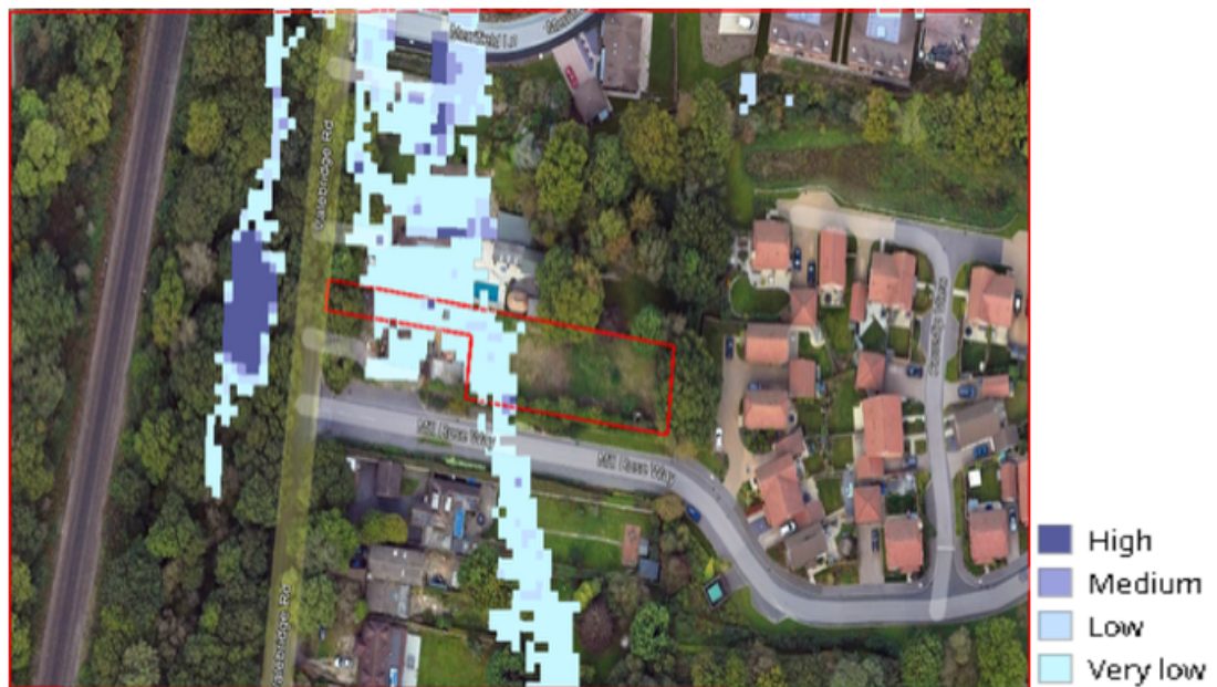
Figure E - Environment Agency Risk of Flooding (0.2m) from Surface Water View
