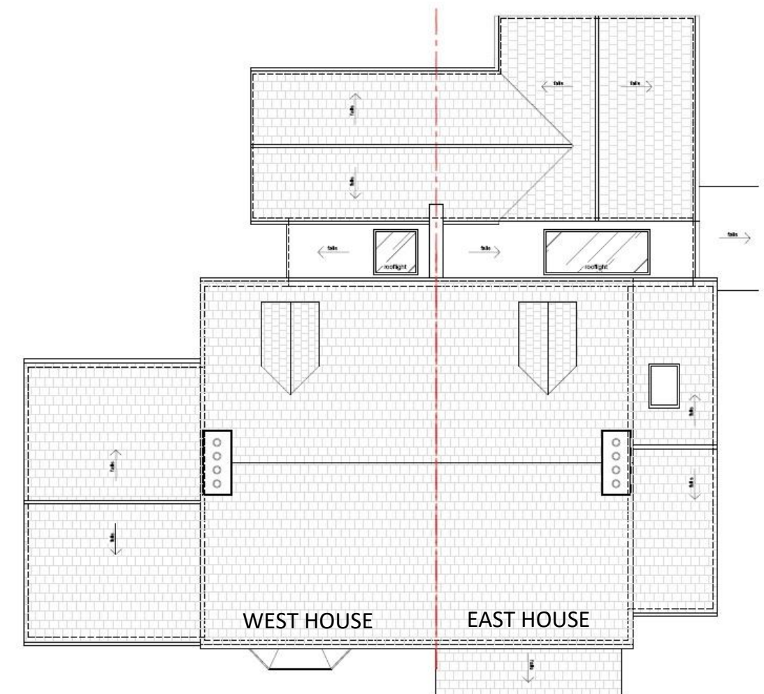
ROOF PLAN SHOWING SUBDIVISION OF BUILDINGS
