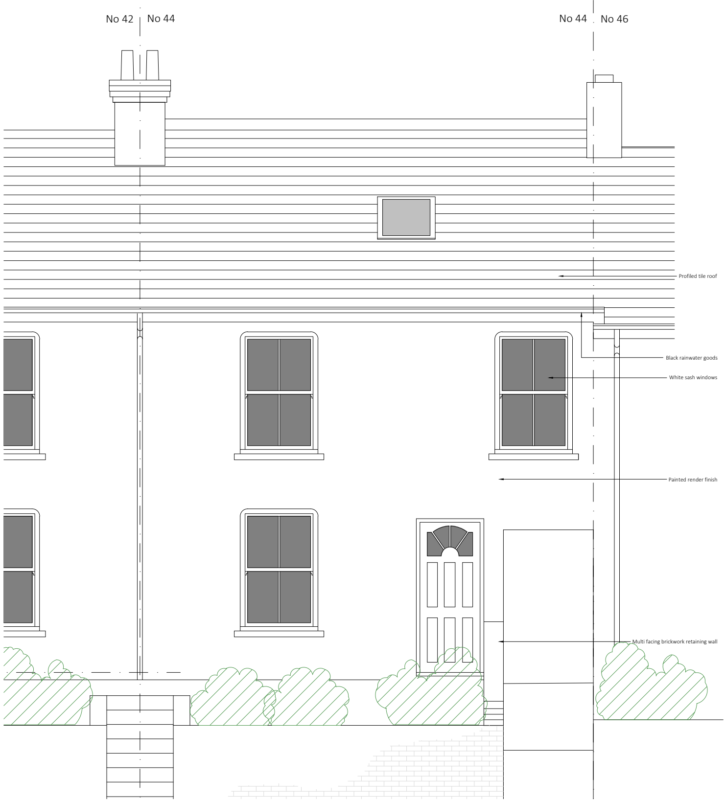
Front (East) Elevation as Existing 1:50 @ A1
