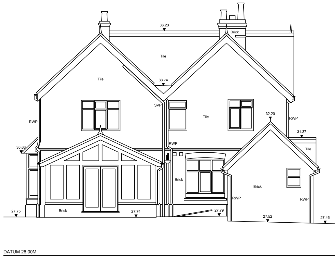
EXISTING WEST ELEVATION
