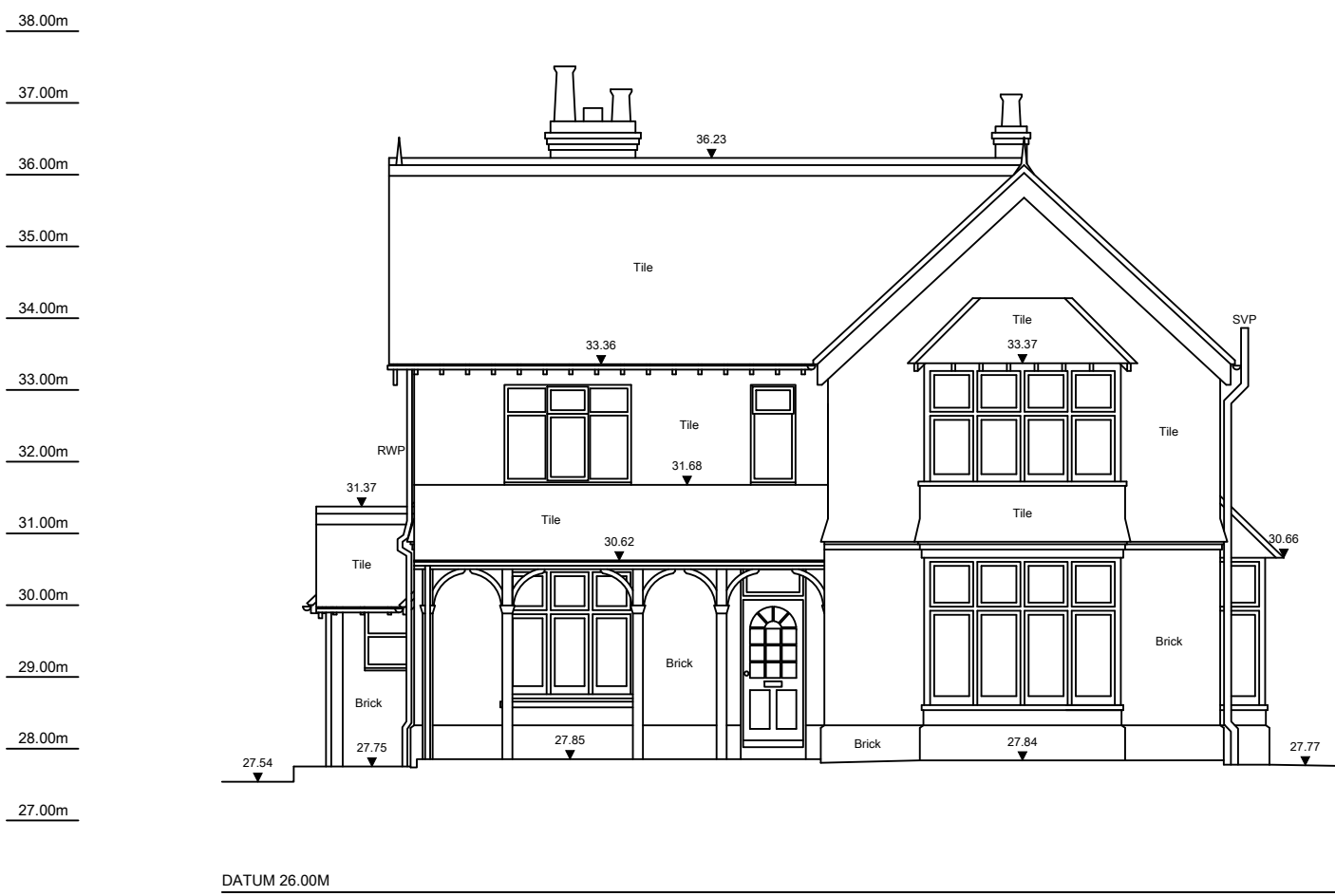
EXISTING EAST ELEVATION
