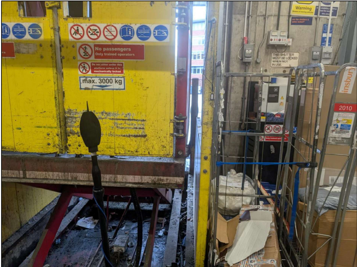
Tail Lift Measurement Position – similar lift motor model to proposed installation (confirmed by lift installer)
