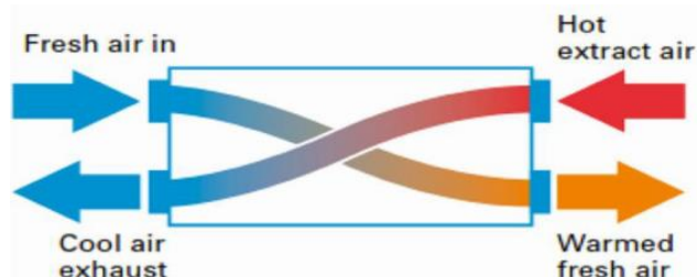
Figure 3.2: MVHR Diagram (Source: www.nfan.co.uk )
