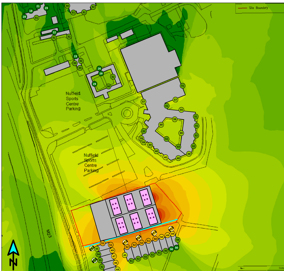
Figure 6.1: 2D acoustic model output of existing scenario + allocated housing
