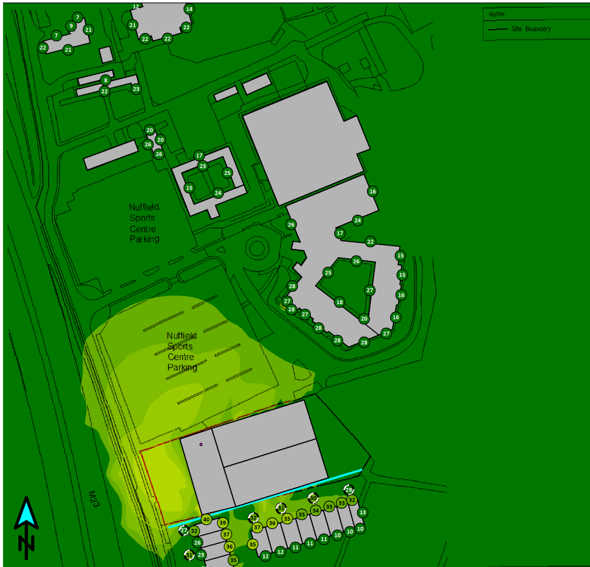
Figure 8.2: Noise map of kitchen extraction system noise emissions (Specific Sound Level calculation)
