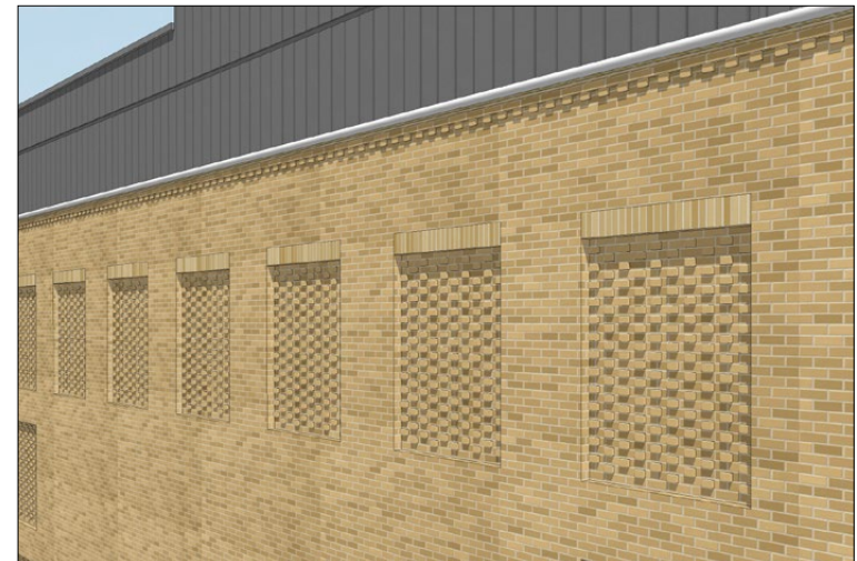
TEXTURED BRICKWORK PANELS TO THE WEST ELEVATION
