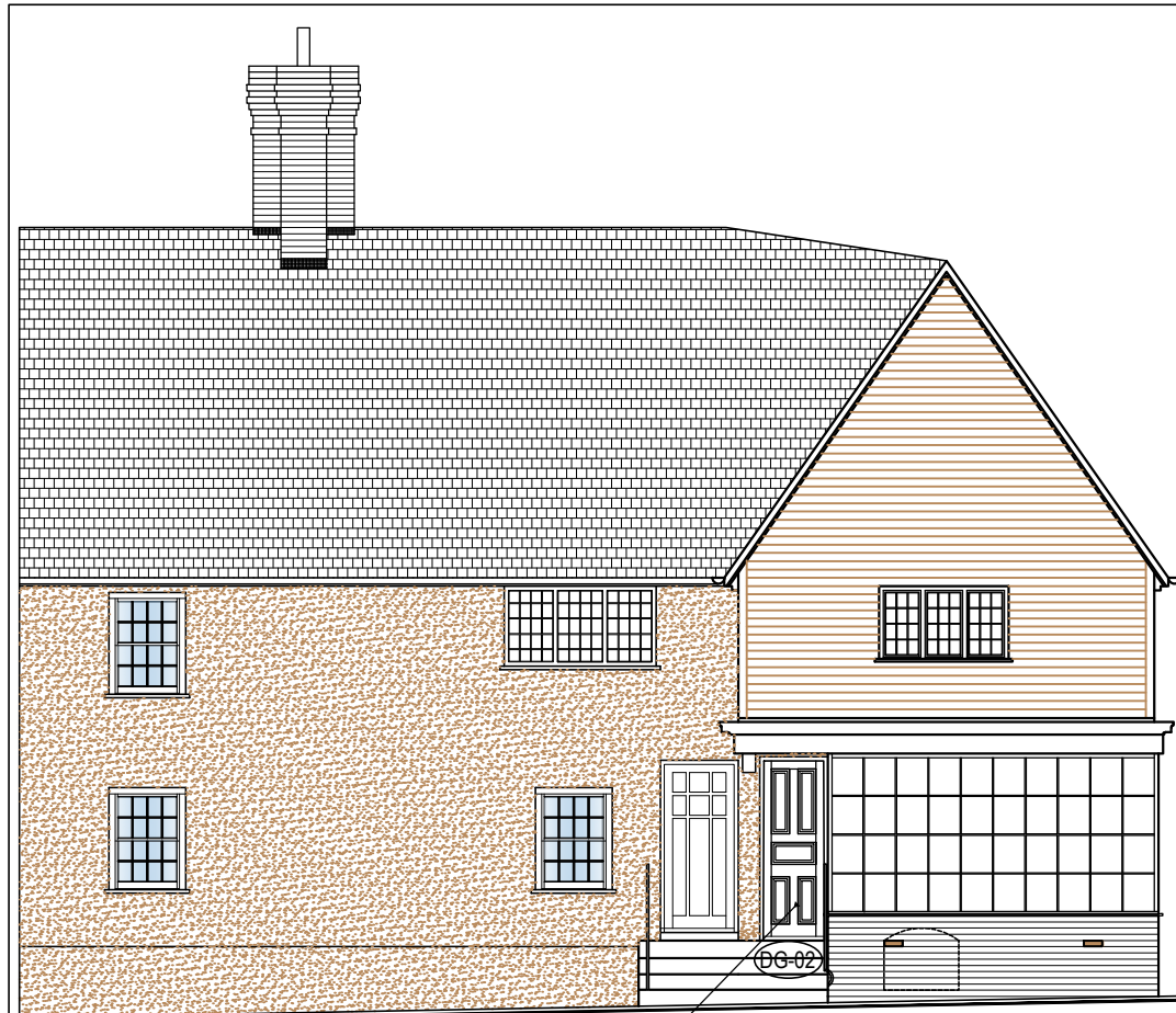
PROPOSED WORKS: FRONT EAST FACING ELEVATION
