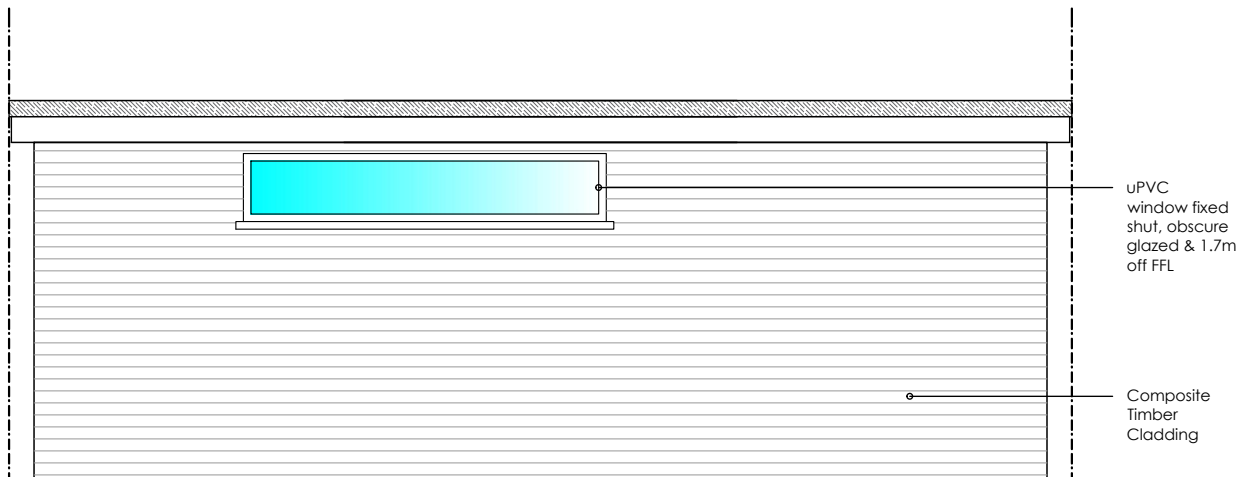
Proposed Rear Elevation Scale 1/100@A3
