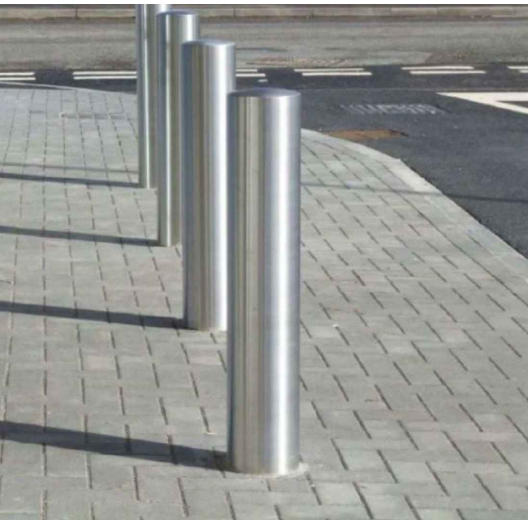
1.2m Stainless steel bollard 1200mm centers
