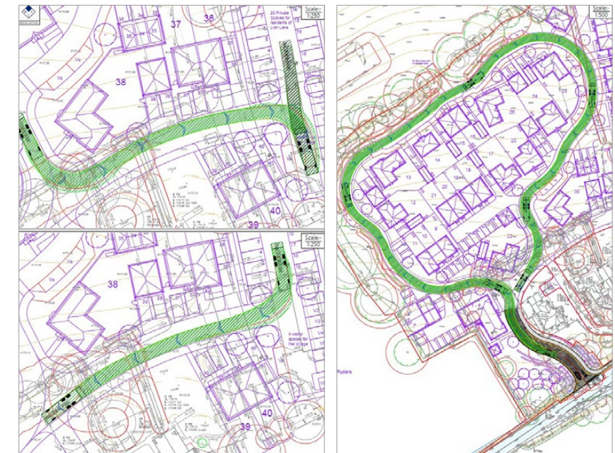
Swept Path Analysis of a 10.5m Refuse Collection Vehicle
