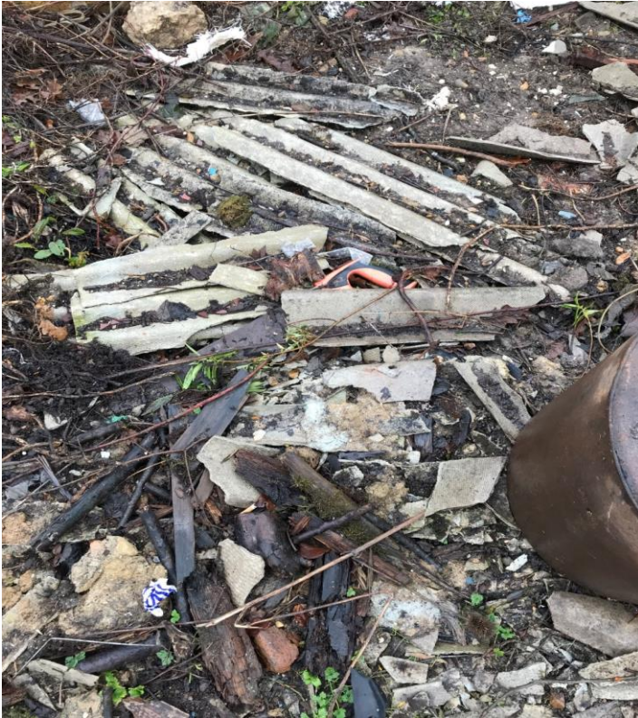
Photograph 9: View of broken potential asbestos containing material in the south of the Site.
