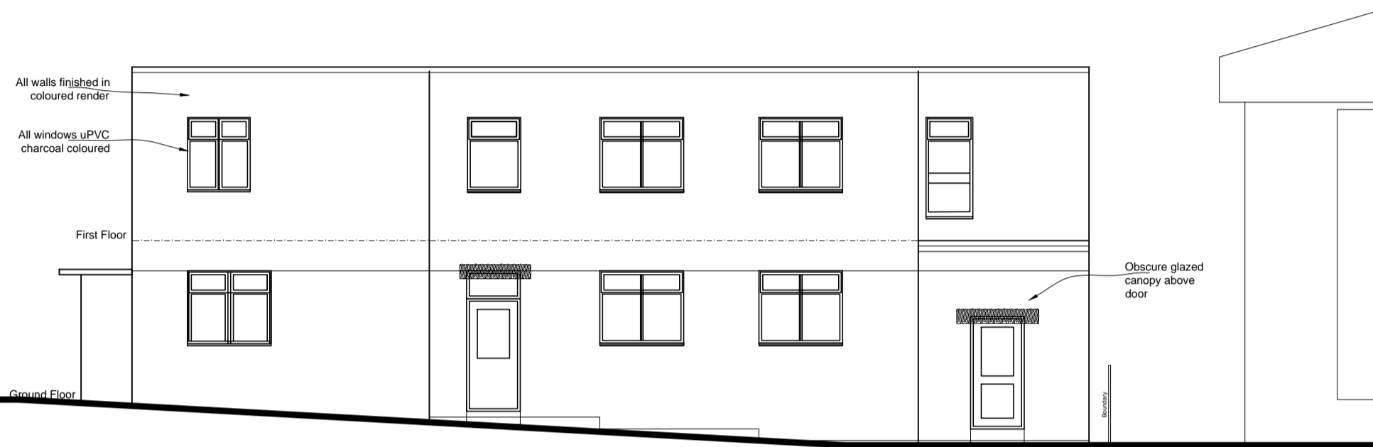
Elevation to Victoria Way - North
