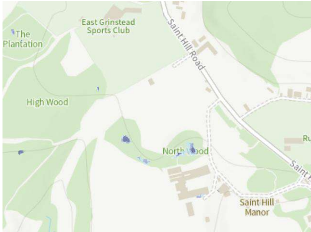
Figure 11: EA RoFSW data showing chance of 600mm water depth during the 2040-2060 surface water event
