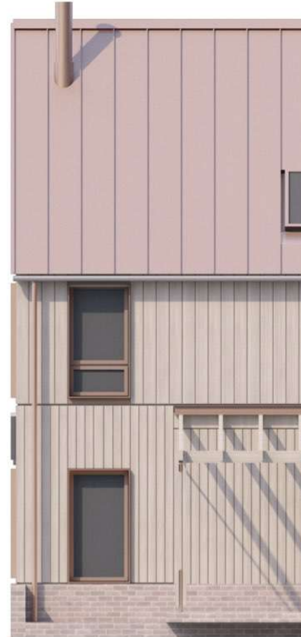
Eave and window detail, down pipe and timber cladding.
