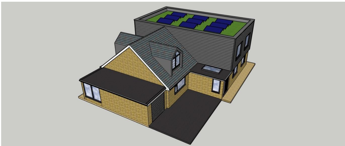
Above: Aerial view – showing green roof with solar panels
