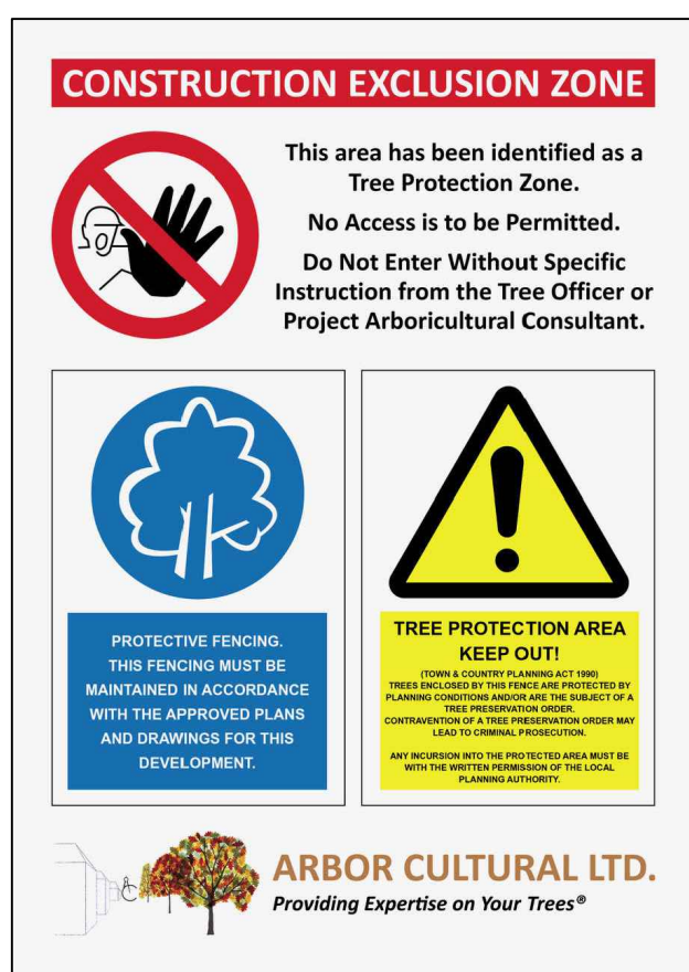
Figure 3 Example of Signage on Fencing
