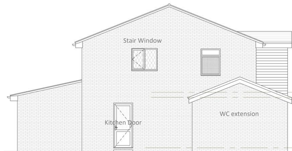
Side Elevation of No.23 illustrating the relationship between the WC extension and rear Kitchen door and Stair window at 1st floor.
