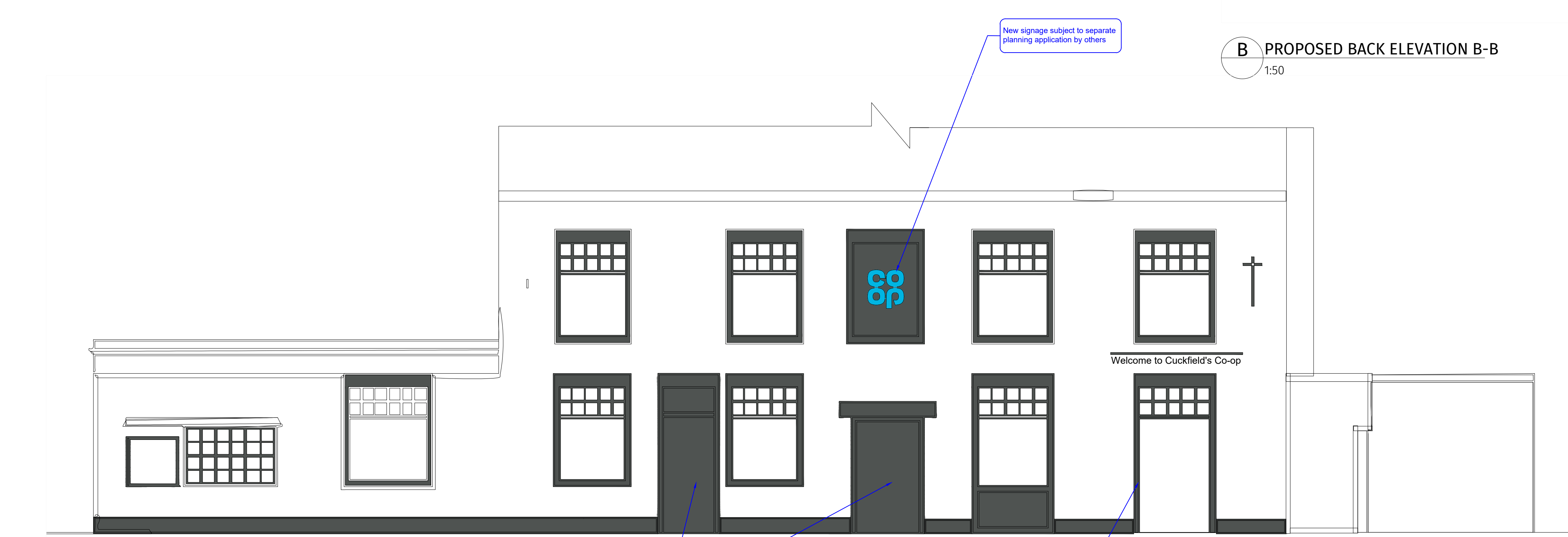
Apply new di-bond panels to 2 x disused windows and doors in Traffic Grey RAL 7043.
