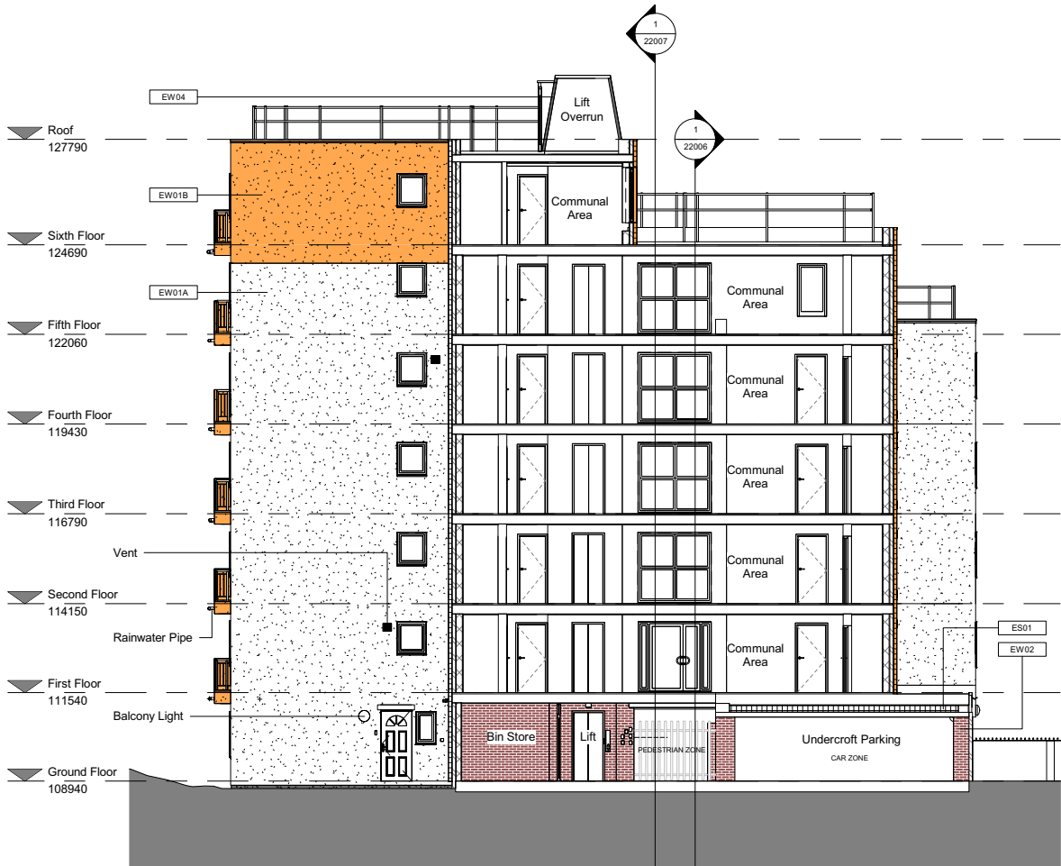
1 | Planning - Existing Elevation Reveal facing North 1 : 100
