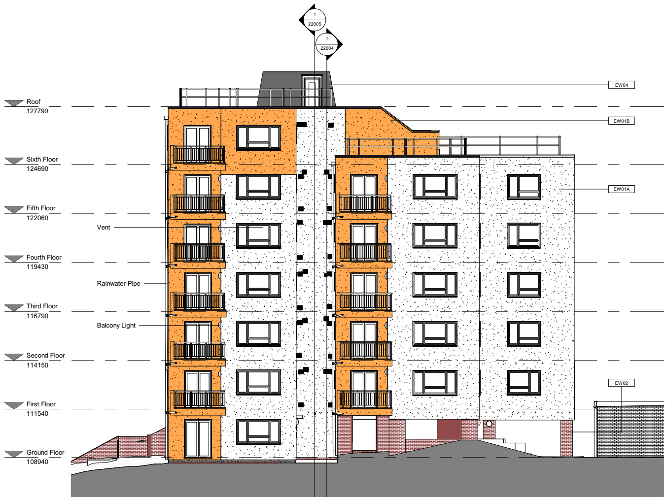
1 | Planning - Existing East Elevation 1 : 100
