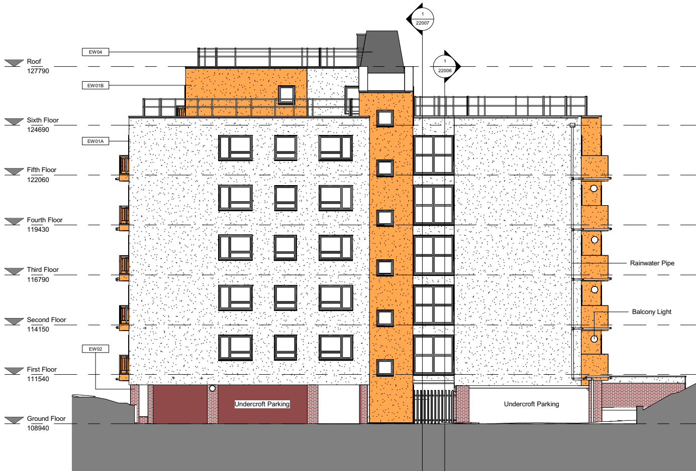
1 | Planning - Existing North Elevation 1 : 100
