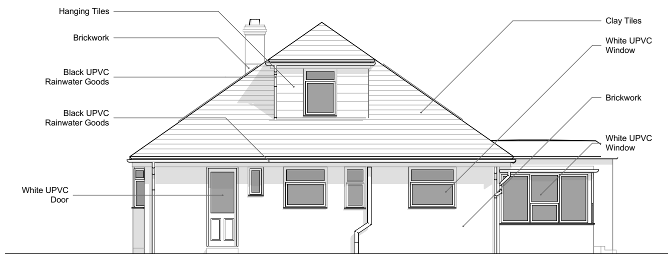
Existing North Elevation
