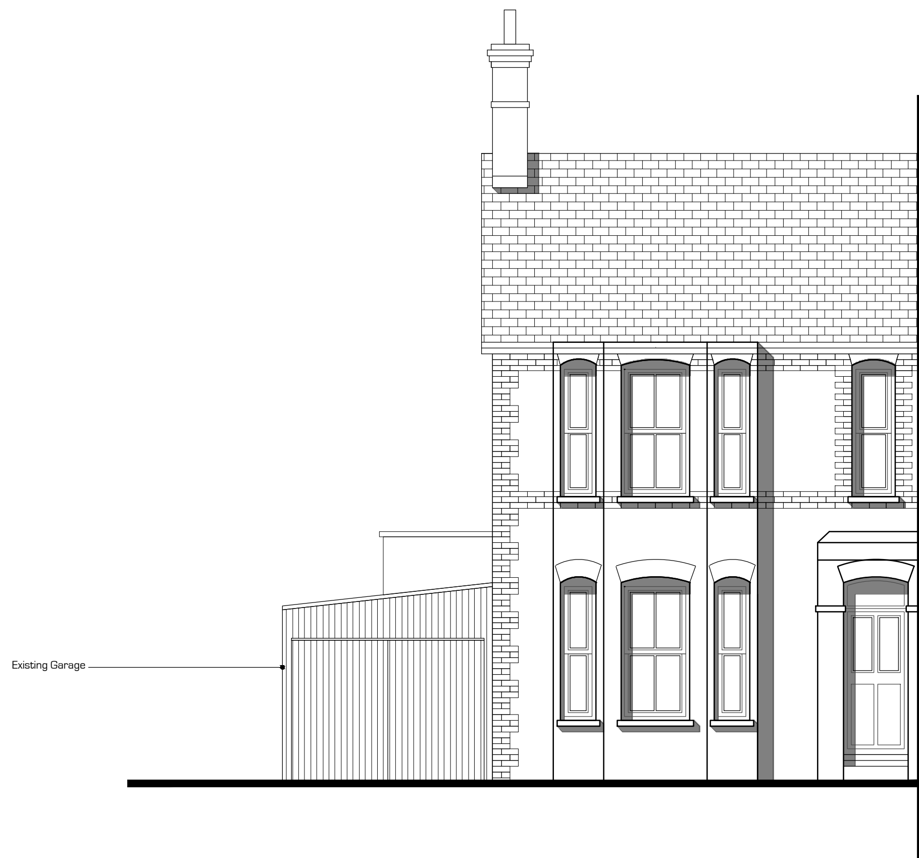
01 Existing Front (East) Elevation 1:50@A1
