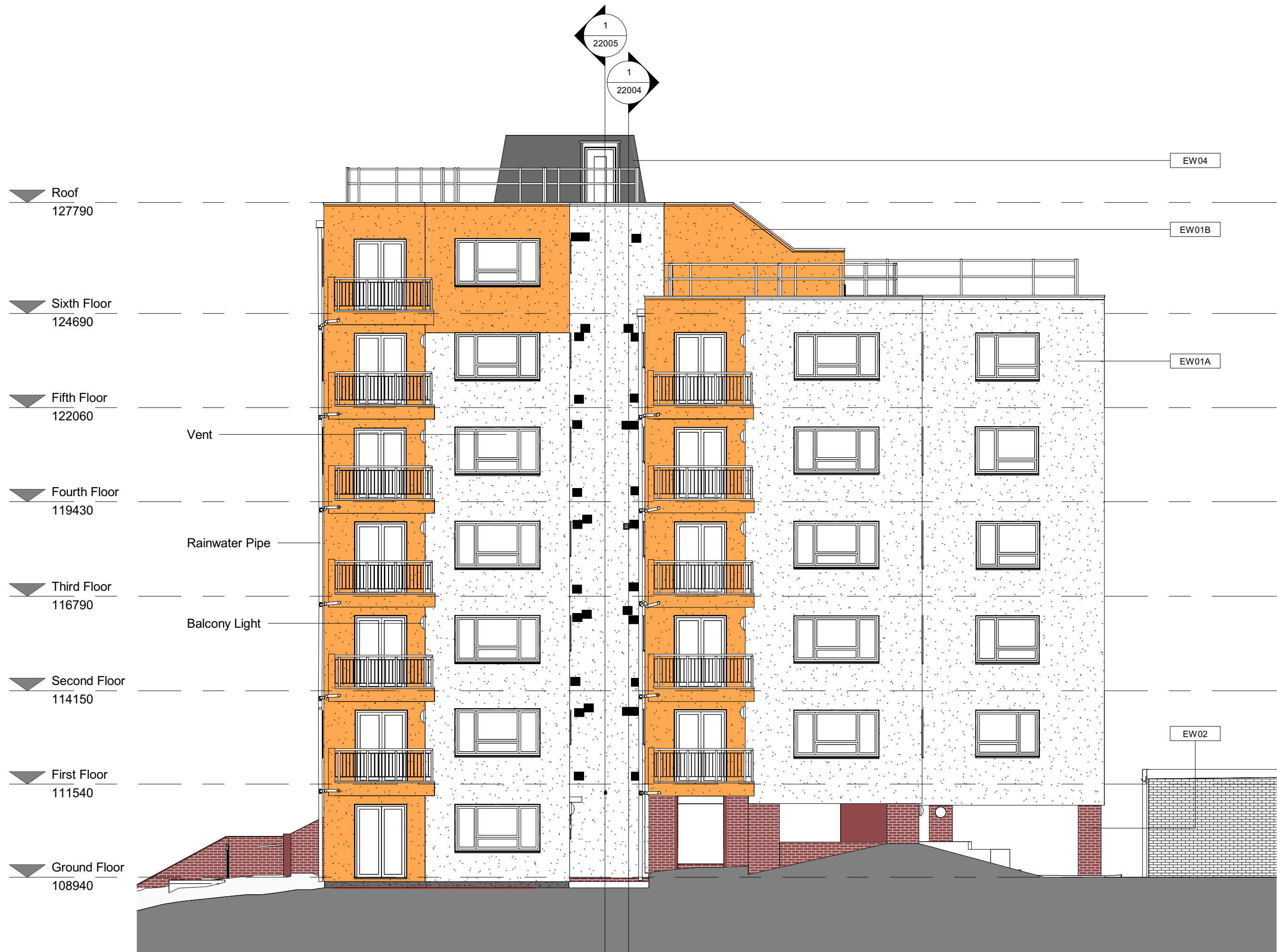
1 Planning - Existing East Elevation 1 : 100
