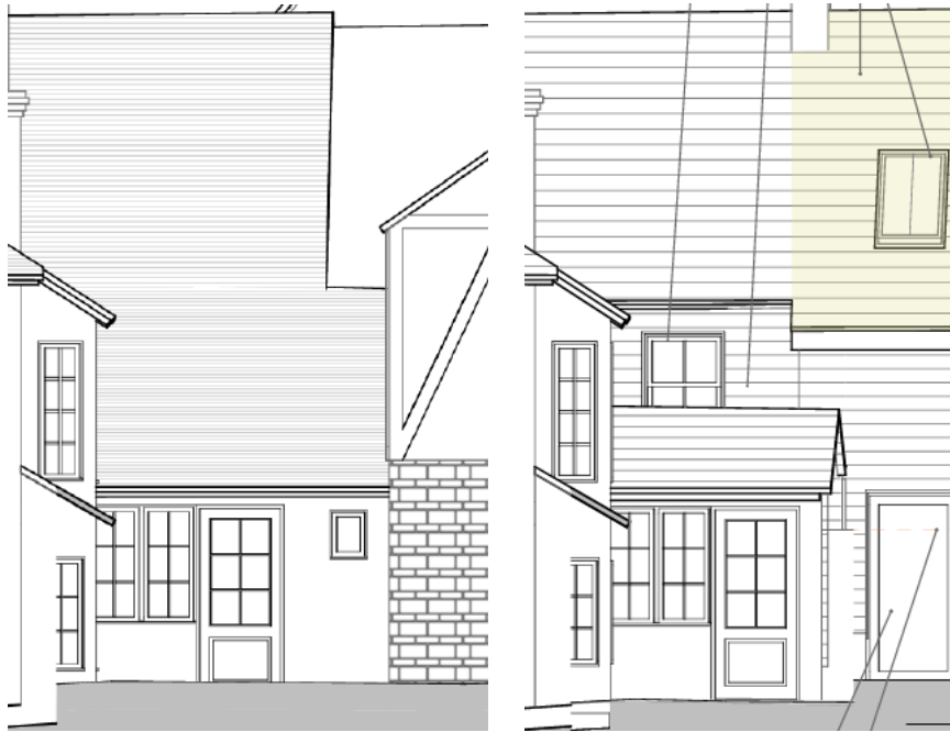
Figure 97 (left): Extract from existing south elevations of The Friary and Somners – showing the modern single-storey rear extension to The Friary, with its mono-pitched roof which continues from the pitched roof of Somners. (See also Figure 36 & Figure 105.)
