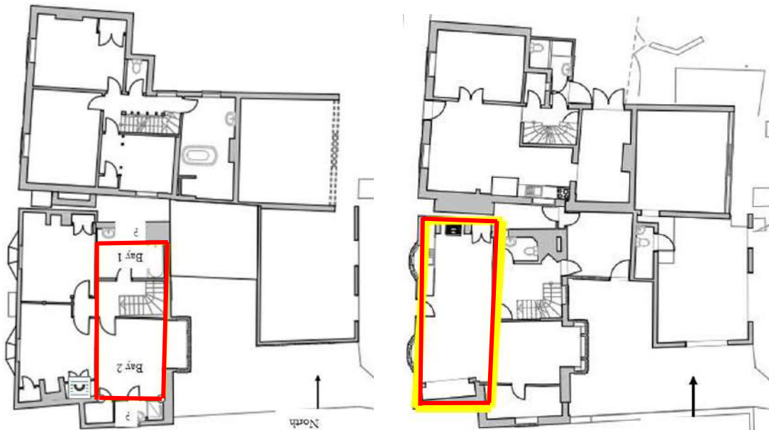
Figure 126 (left): Phase D1 – Late 18 th /early 19 th century. The Friary : Roof raised higher over Phase A and B chambers. Wall painting imitating wallpaper.
