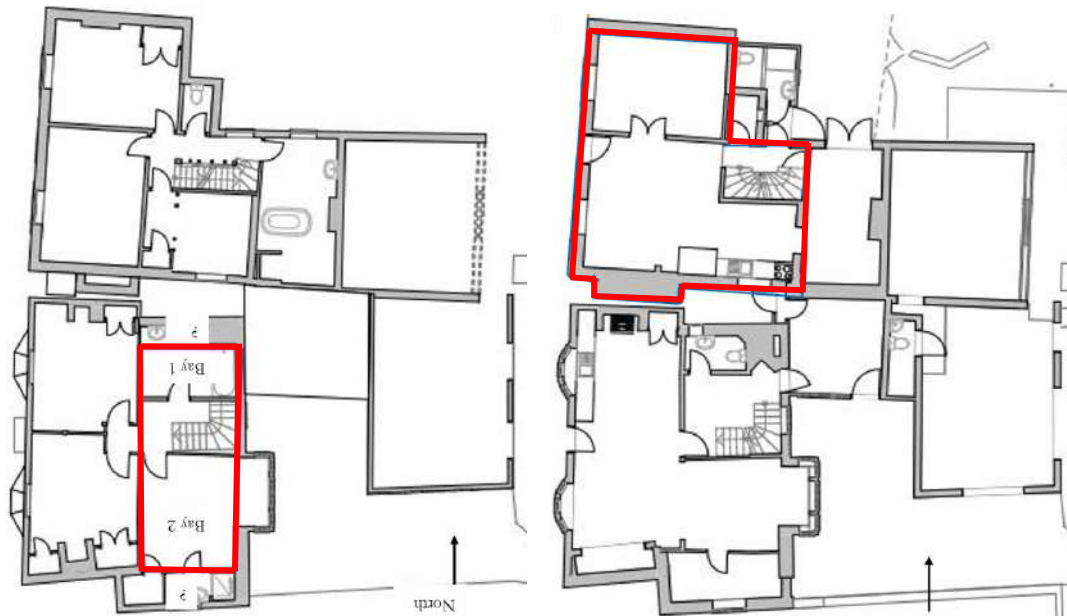
Figure 122 (left): Phase A – Mid-16 th to mid-17 th centuries. The Friary : Two or more bays built with a smoke bay or open hall. Clapsed side purlin roof and small panel framing.
