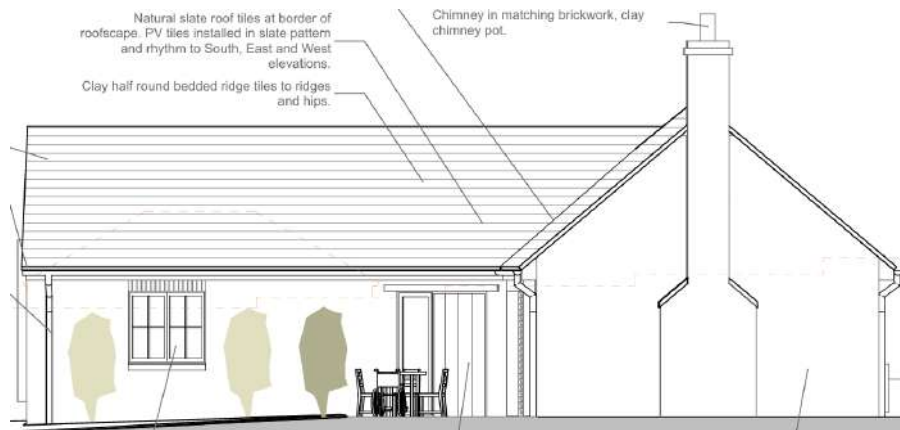
Figure 104: Proposed side (east) elevation of Dumbrells.
