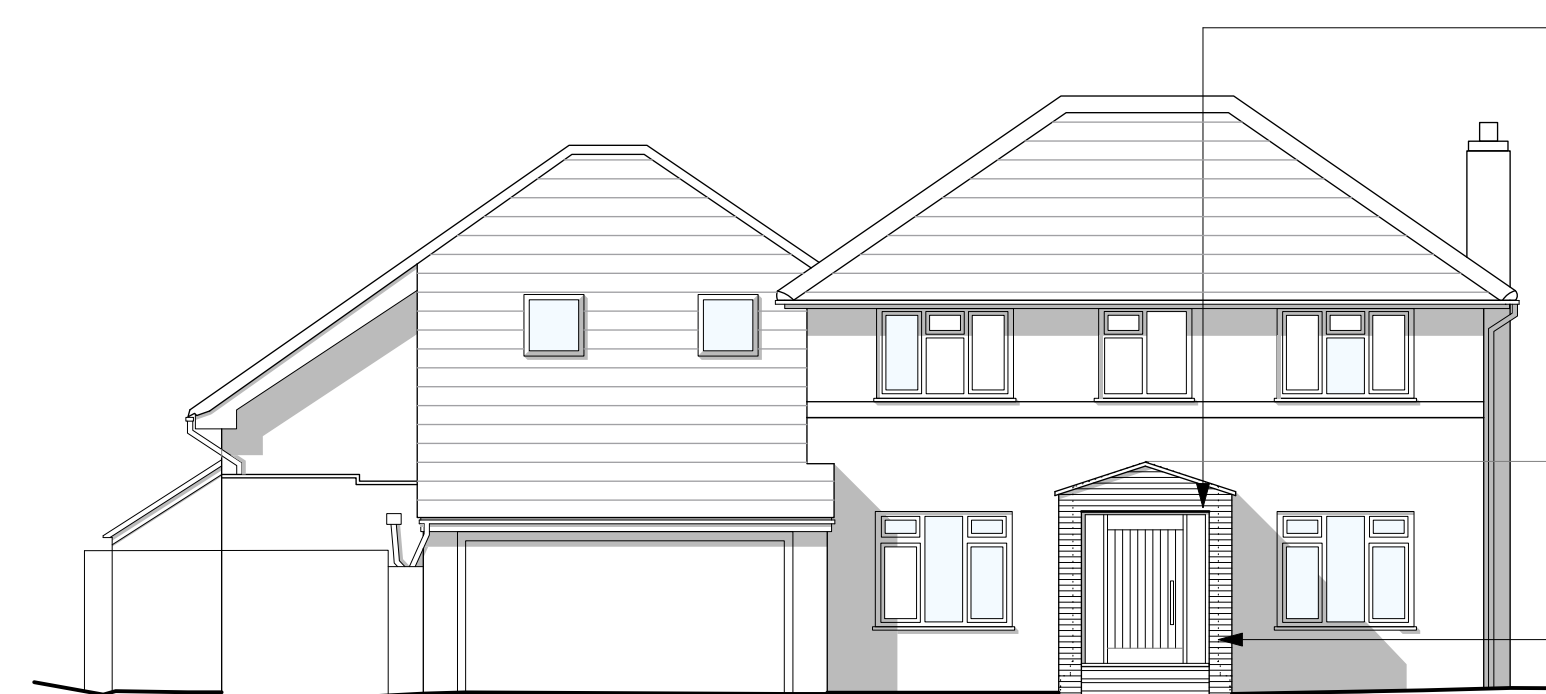
Front Elevation - showing new porch.
