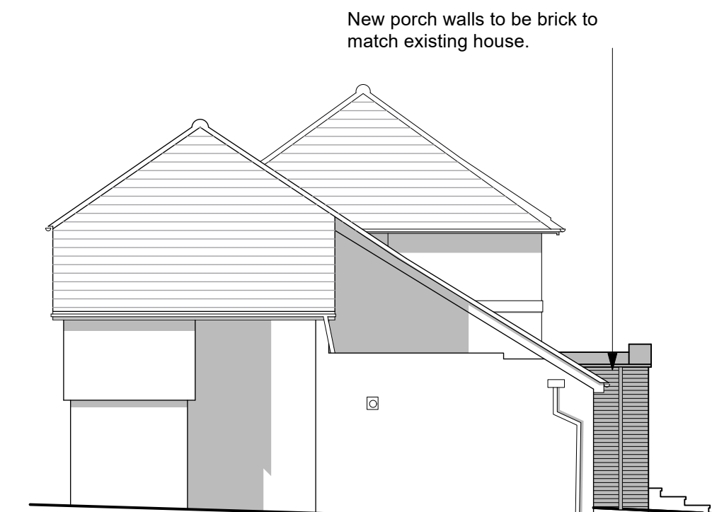
Side Elevation - showing new porch.
