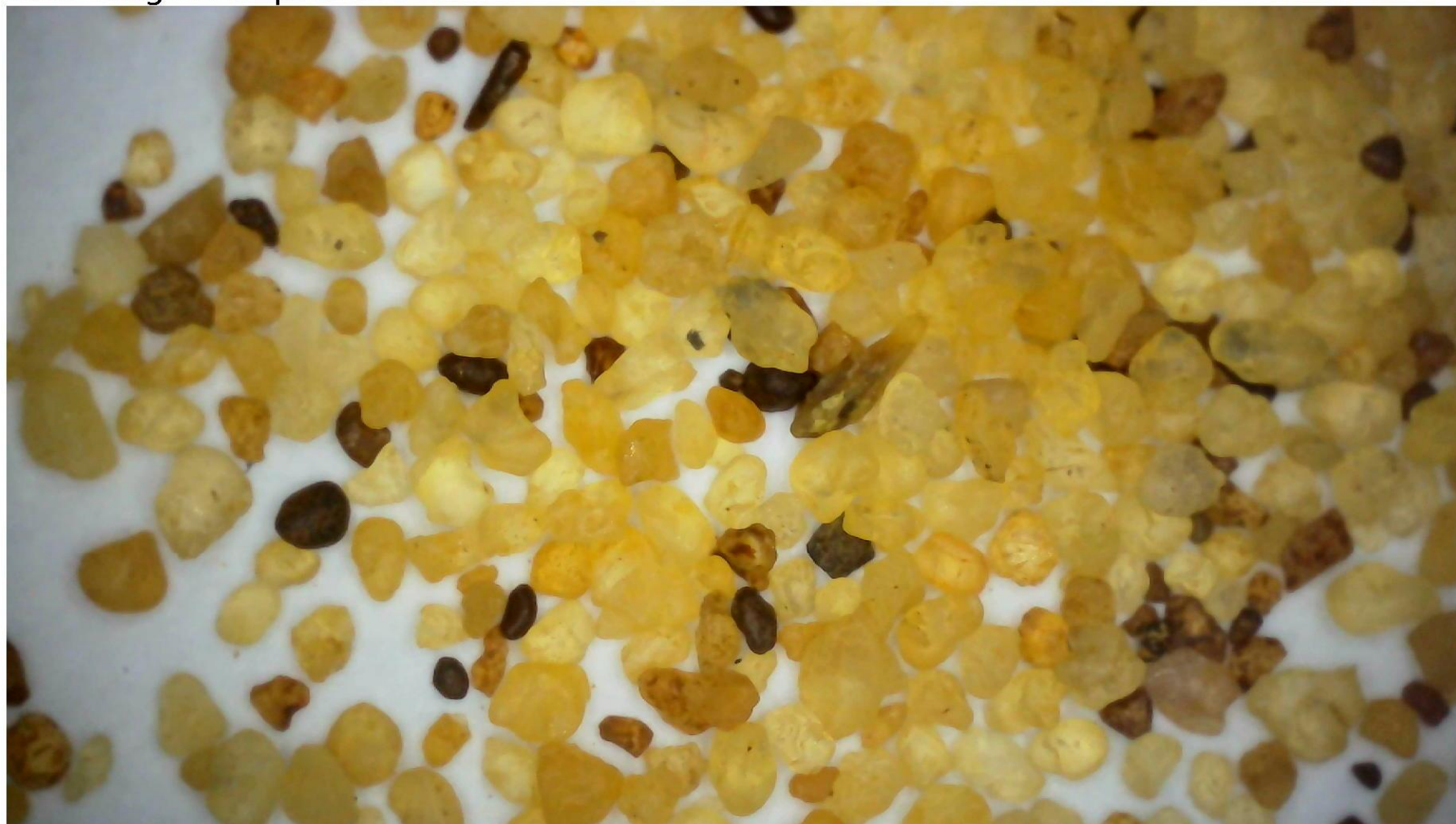
Stabilising Infill - picture
