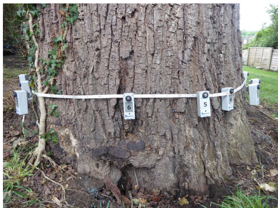
Figure 2. East side of trunk - sensors indicate height of test.
