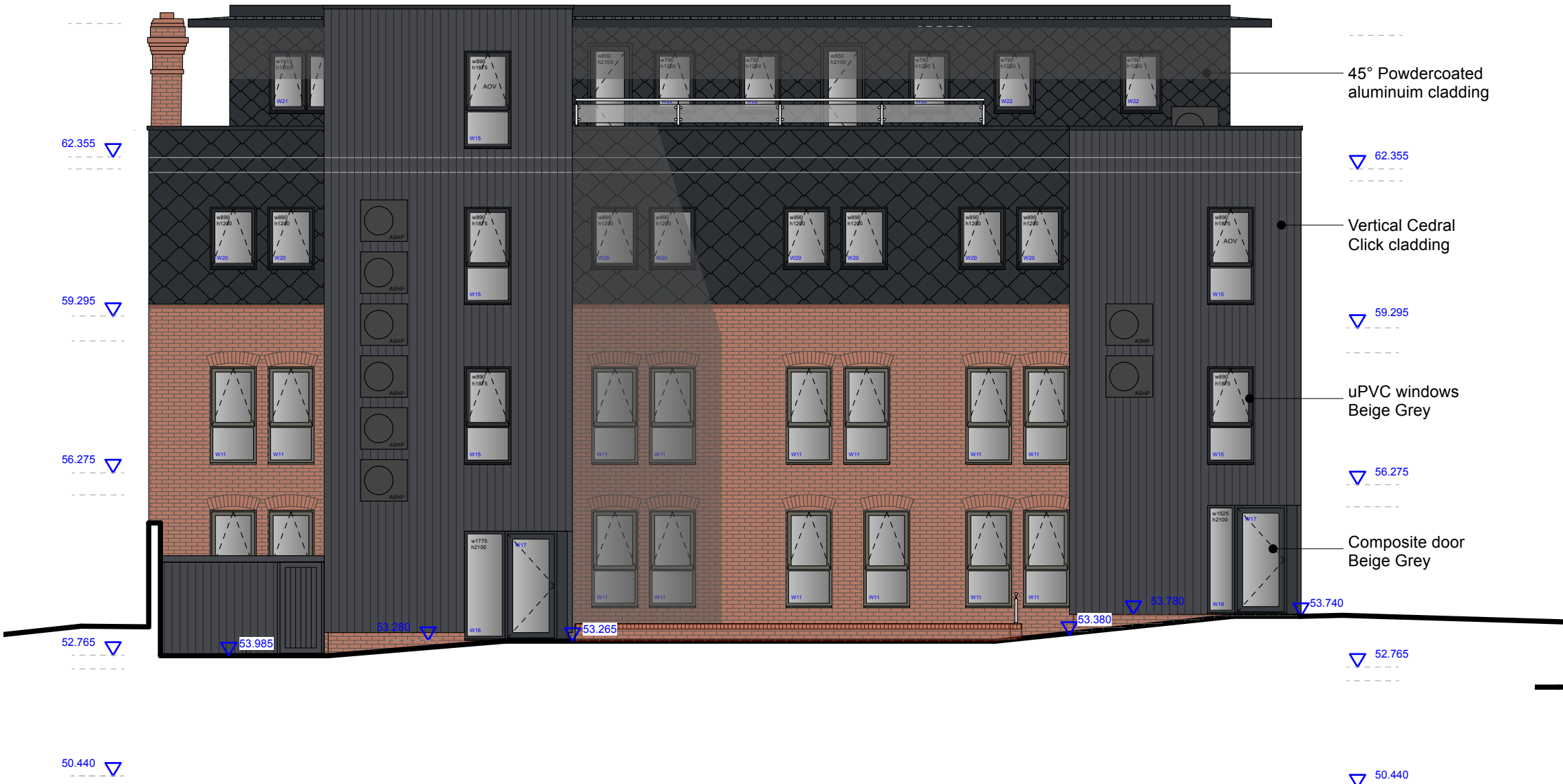
West Elevation (Rear)
