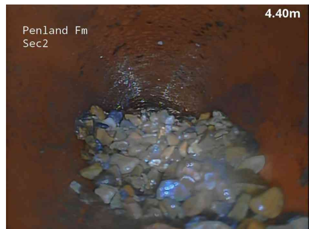
4, 00:00:28, 4.50 m Survey abandoned, Camera compacting shingle
