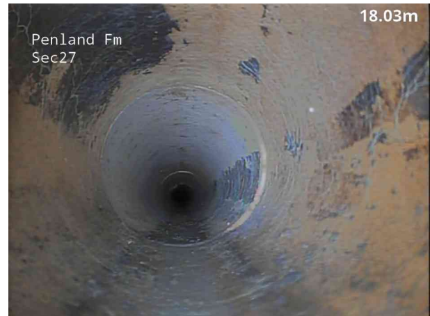
10, 00:01:48, 18.20 m Roots, fine at joint, finish
