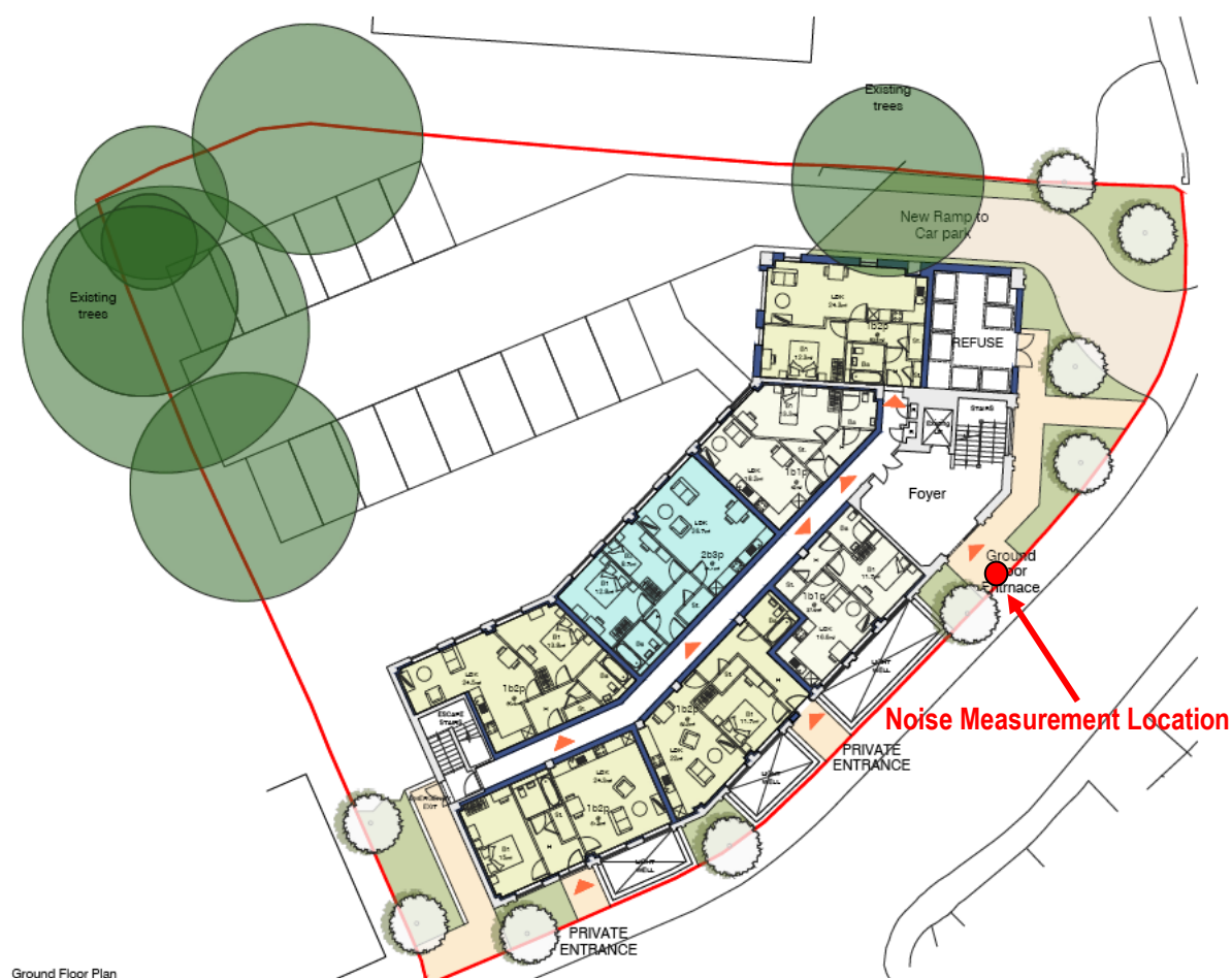
Figure 4.1: Noise Measurement Location & Proposed Ground Floor Plan
