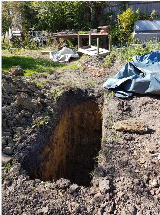
Fig 1 - Soakaway test pits in 2019
