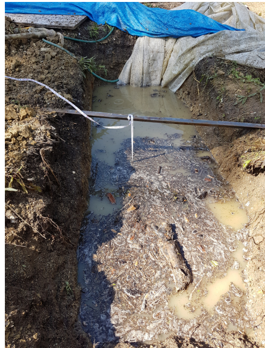
Fig 1 - Soakaway test pits in 2019
