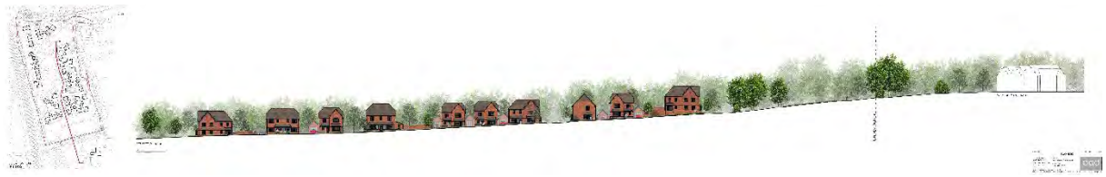
Figure 6.1. Section through the site showing the relationship with Wickham Farmhouse and the use of the topography.
