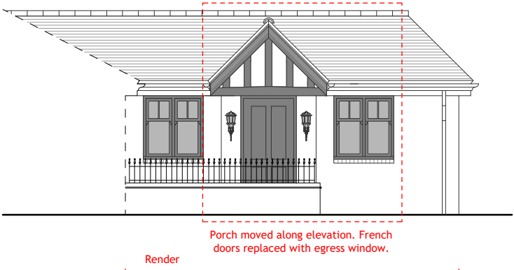
South-West Elevation (Plot 06)
