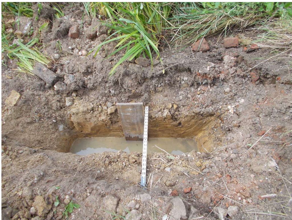
Photo 6: Percolation Test Pit PTP 2.
