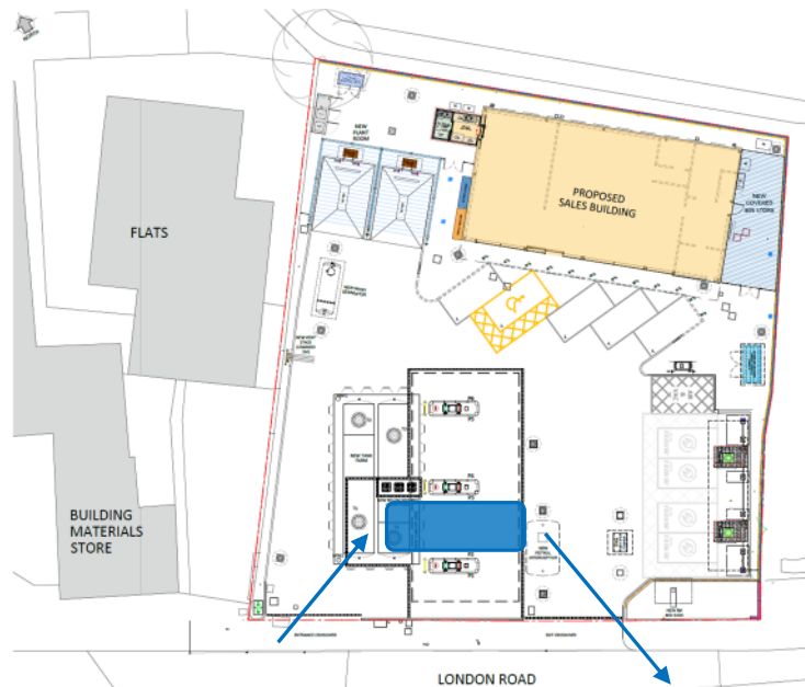
Figure 4: Illustration of fuel delivery location and manoeuvre
