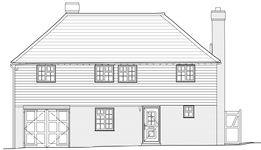
4 Coach House & Shed - Existing East Elevation Scale: 1:100
