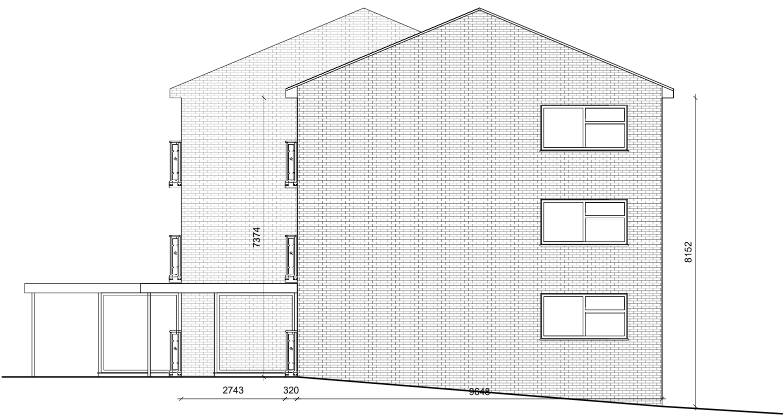
Side (east) elevation 1.100
